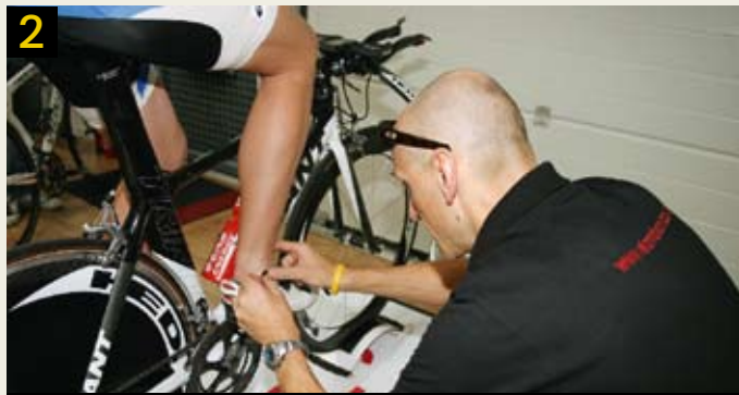
2 Having warmed up and calibrated the turbo, key anatomical landmarks on Tim's feet, ankles, knees, hips, shoulders, elbows and wrists are located and marked with a sticker.
