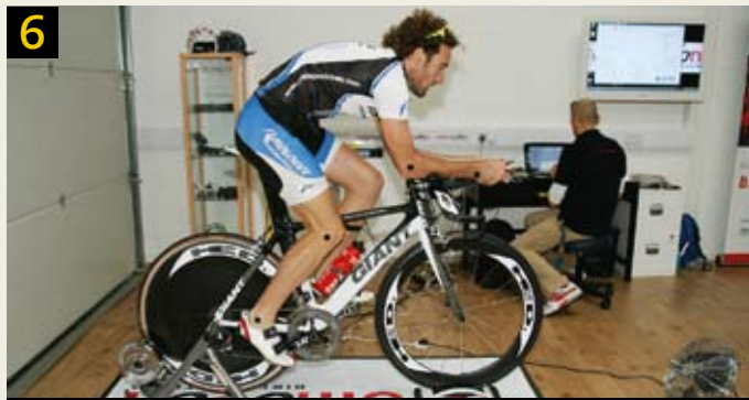
6 Tim re-rides the test in the new position, giving feedback all the time. John records and analyses the data. Both heart rate and perceived exertion are lower for the same wattage compared to Tim's original position.
