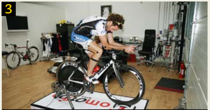
3 Tim has the LED harness fitted and then progressively builds up to a sub-threshold effort. The 3D camera is constantly logging data throughout.
